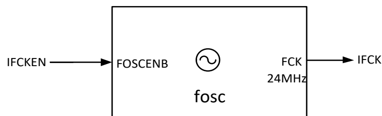
Figure 23-1 Input/Output of Internal Fast Clock
