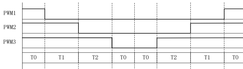
Figure 14-8 Continuous SVPWM Output Waveform
