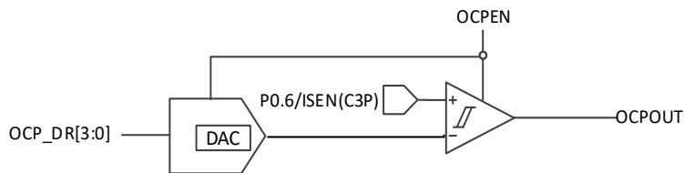
Figure 20-2 Input and Output Signal of OCP
