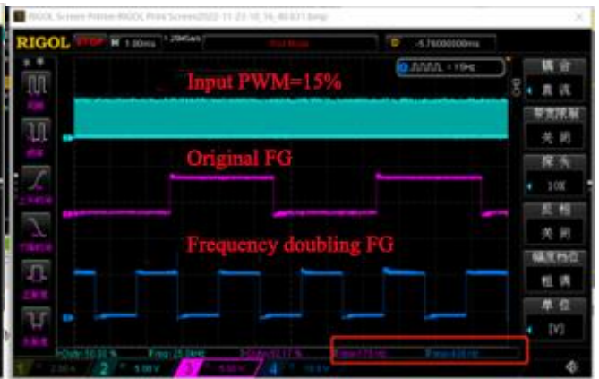
Figure 3-30 Virtual FG example two
