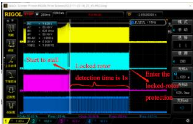
Figure 3-41 Lock detection example
