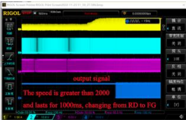
Figure 3-36 Switching FG at high speed example one
