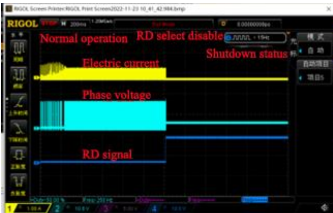
Figure 3-31 RD signal example one
