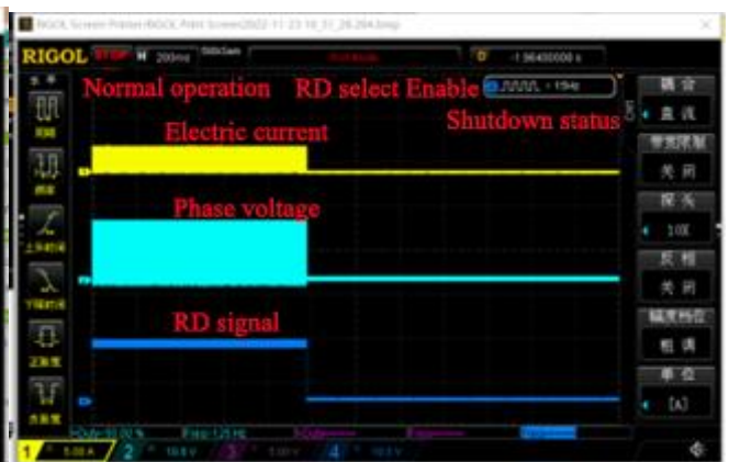
Figure 3-32 RD signal example two
