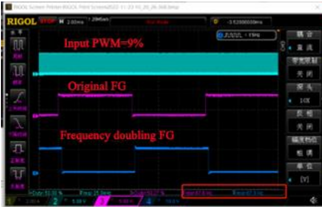
Figure 3-29 Virtual FG example one
