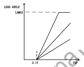
Figure 3. Phase Control Setting Example 1, LA<sub>MIN</sub>=0; difference LA<sub>SKEW</sub>
