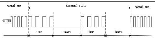
Figure 5 Lockup Protection and Automatic Restart
