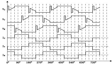
Figure 2 Voltage and Current of BLDC(120°)
